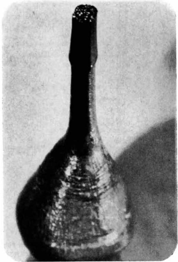
Fig. 2. Zinc single crystal with hexagonal geometry grown in a macrosonic field (25 kc).
